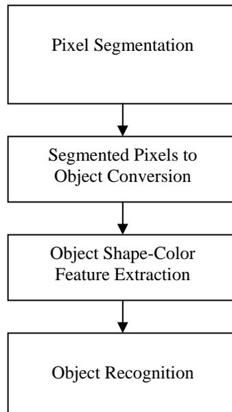
Figure 3: Image analysis to extract the quantities of the various trash constituents.
