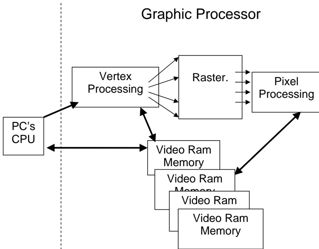
Figure 6: Processing flow using a GPU processor
