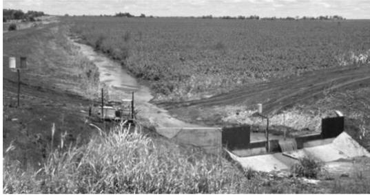
**Figure 2. Instrumentation used to measure runoff, erosion and pesticide movement in the dryland study.**
