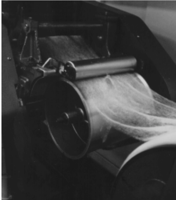
Slide C-1: Mini-carding and collecting system.
