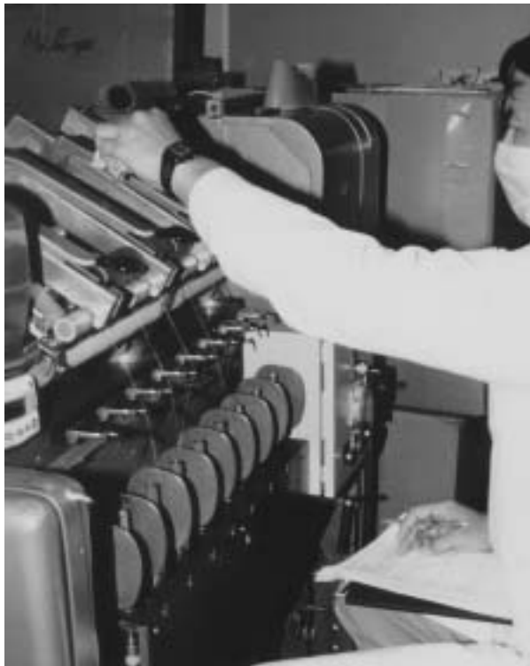
Slide C-5: Ring spinning frame during a stickiness observation phase.
