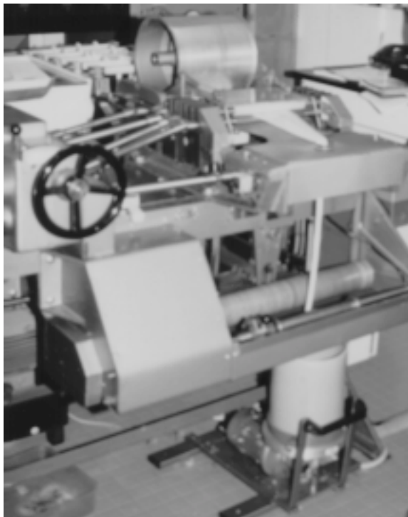
Slide C-2: Drawing-frame and collecting system in cans.
