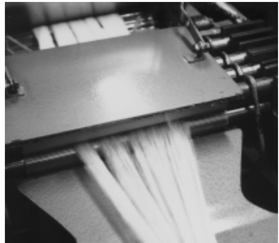
Slide C-4: Drafting zone of the drawing frame.
